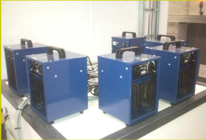
Energy dissipation (1-12 kWe)
